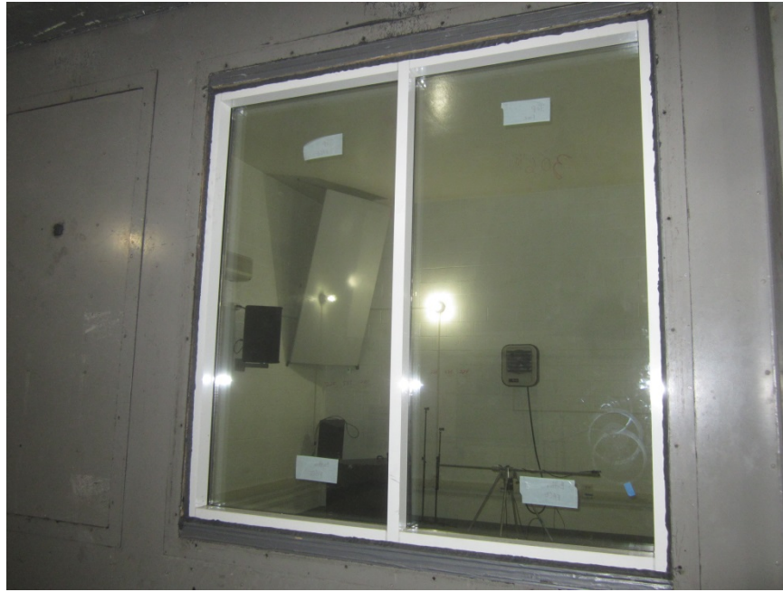
Receive Room View of Installed Test Specimen
